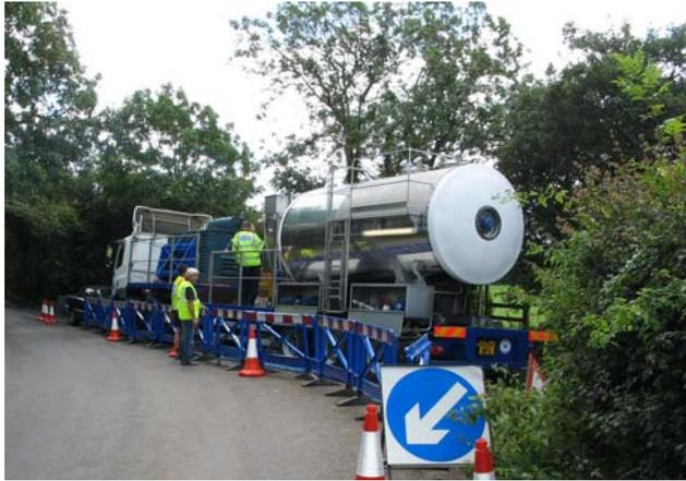
Figure 9 The ice-pig delivery lorry ready to undertake a live trial
