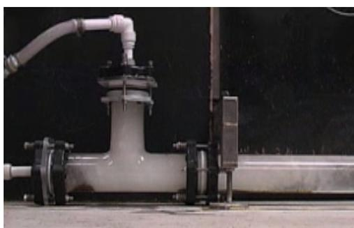
Figure 5 The ice pig has entered the system from the small 22mm pipe at the top of the T and has formed a viable pig in the horizontal 75 mm internal diameter pipe.
