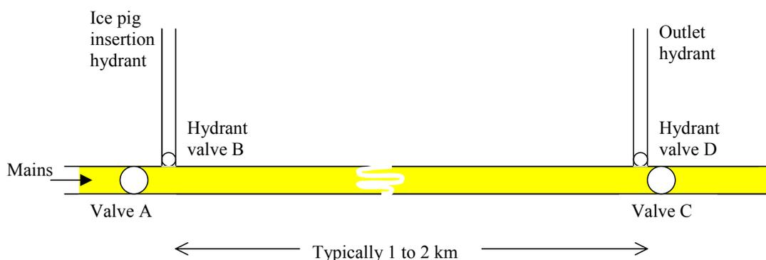
Figure 10 Schematic of the ice pigging procedure
