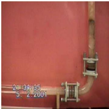
Figure 2, 90-degree bend joining a horizontal and vertical pipe. The sand was originally at the bend at the bottom of the vertical pipe. The figure show the sand as it is being transported up the vertical section.
