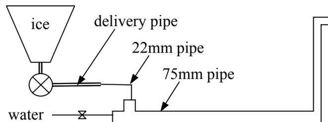
Figure 4. Schematic of experimental rig.
