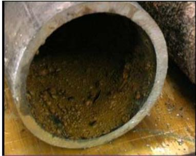
Figure 6 Cut out iron pipe from a 4 inch trunk main. Note the corrosion and rough internal surface.
