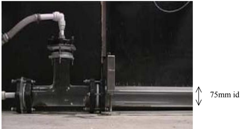
Figure 3 75 mm diameter pipe with a T feed from an 18mm diameter delivery pipe.
