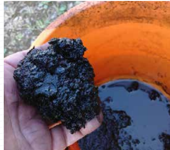
Sludge deposits that were cleaned from inside the pipe walls.
