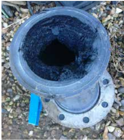
Sludge deposits that were cleaned from inside the pipe walls.
